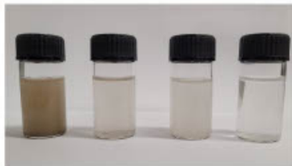
Turbidity samples, from left to right: LMS-1 1:100, LMS-1 1:500, LHS-1 1:100, LHS-1 1:500
