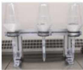
Figure 2: Test-setup water in lunar regolith (saturation occurs at around 16%).
