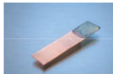
Electrodeposited Iron on copper substrate Electrolyte: IL-TriCl with dissolved regolith simulant
