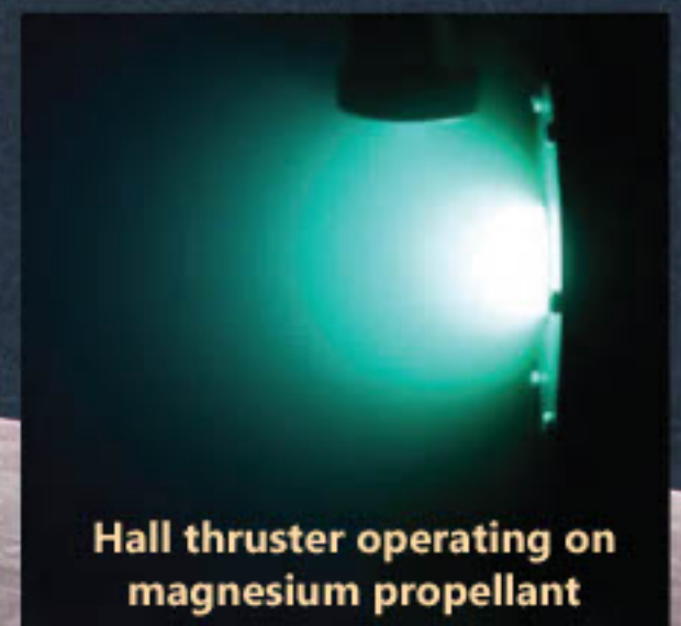
Hall Thruster set up to use propellants stored in solid form
