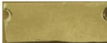
Figure 1. Pitting and cracking shown in color differences in returned portions of Surveyor 3 [1]
