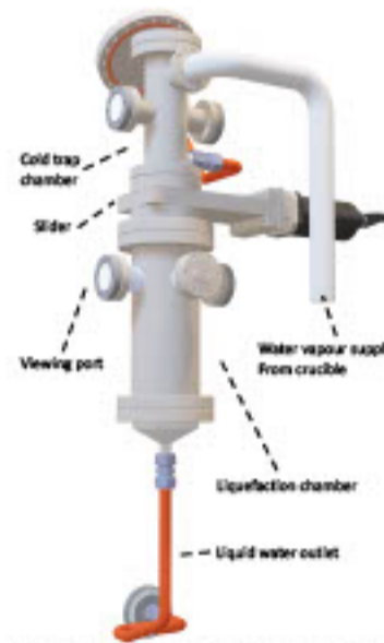
Figure 5: Model of the cold trap and liquefaction.
