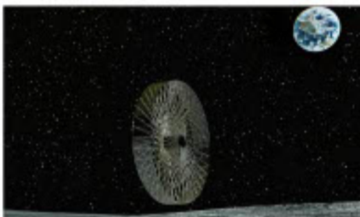
FIG 6: OPLONAS approaches tangentially. Pre-spins to achieve smooth contact
