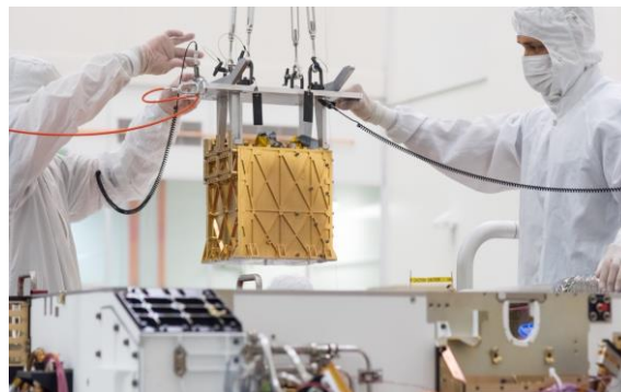
Figure 1: MOXIE being lowered into the Perseverance Rover
